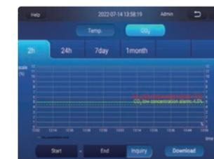
Real-time display of operation data & real-time display of temperature, for CO<sub>2</sub> concentration and O<sub>2</sub> concentration, and the data during the culture cycle can be viewed at any time.
