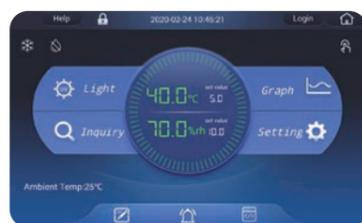
The intelligent 10-inch touchscreen controller is easy to operate and sensitive to touch, even in rubber gloves. The PID control algorithm ensures the accuracy of temperature control
