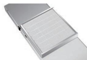
The optional HEPA high-efficiency filtration system combined with the unique air duct circulation design can continuously filter pollutants (biological pollutants and suspended particles) in the cabinet, ensuring that the incubator can reach the ISO class 5 clean room within 5 minutes after the external door is closed, which is equivalent to the class 100 environment of the 209 E standard of the united states
